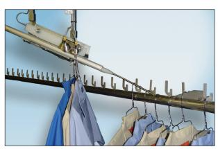
A "cam style" auto-loader for the pendant conveyor systems is an ideal addition anywhere high volume is needed. The auto-loader is fed by a ten foot stainless steel twist conveyor to provide a constant supply of garments. A proximity sensor detects the presence of a hanger on the cam which opens the solenoid to actuate an air cylinder feeding the garment to the conveyor.
